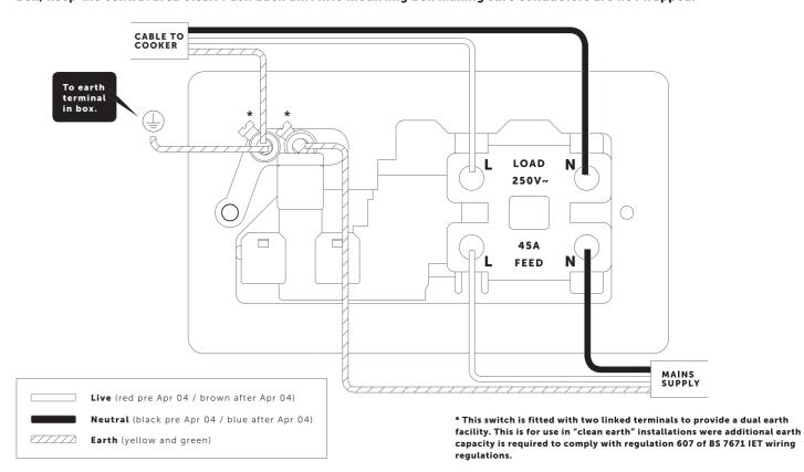
Use a cross head electric or manual screwdriver to fit the screws until tight.\*
